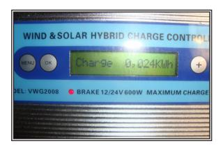
Energy from wind and solar are controlled by a hybrid charge controller. Up to now were 130 kW on electricity produced, enough to supply our pumping system.
