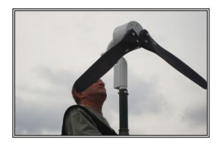
The turbine is driven by wind power at 0,3 kW charge potential and feeds a battery system with electrical energy.
